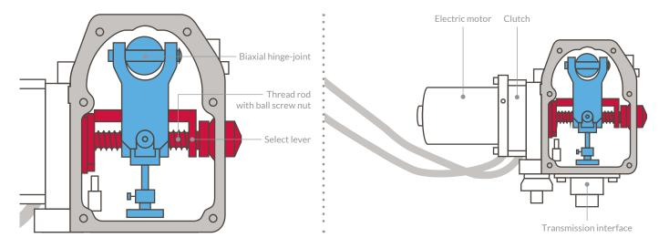
A ball screw nut performs SHIFT, a select lever performs SELECT operations, both moved by the same motor. KSK's One-Motor One-Clutch Electric Transmission Control is actually an innovative simplification of current transmission control systems' construction design.
